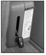
Pull up on the release lever, labeled 1, located on the rear of the seatback and push the seatback forward.
